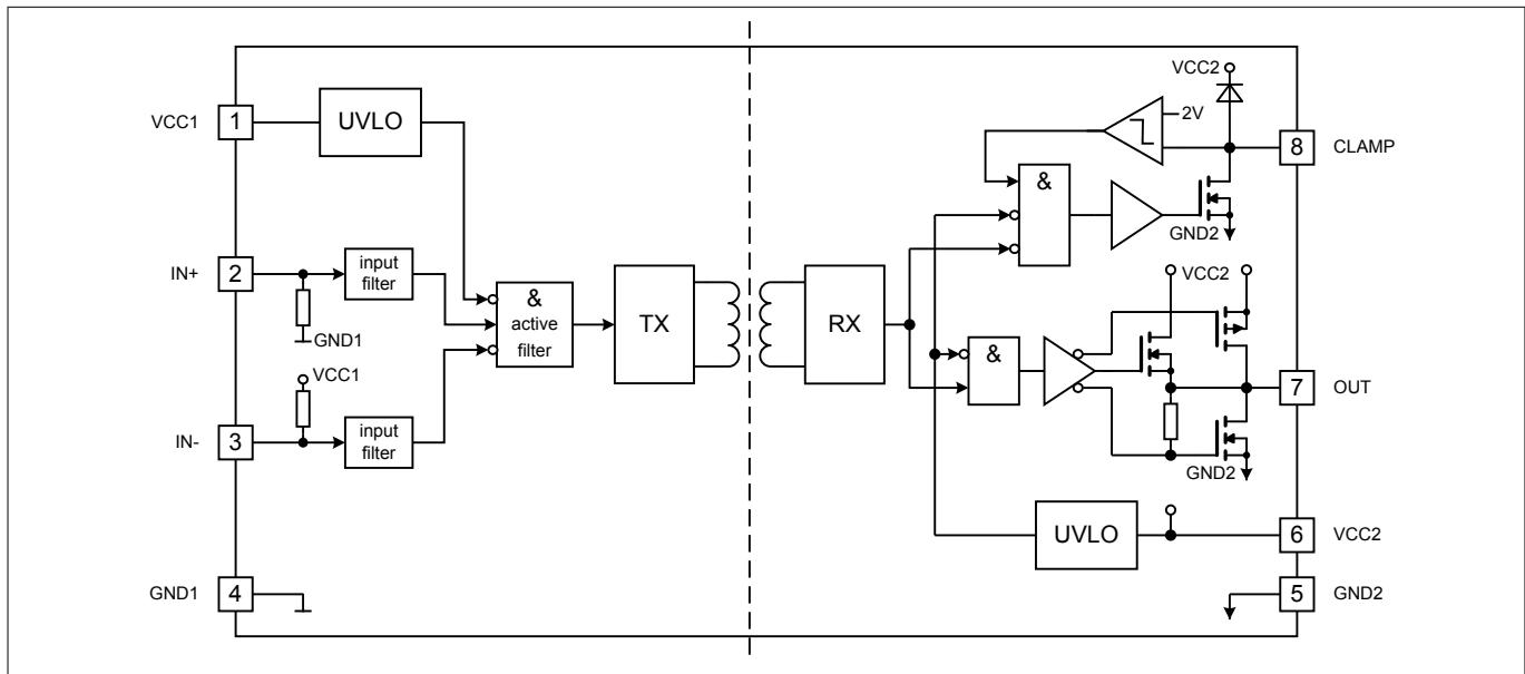
Figure 2 Block diagram
