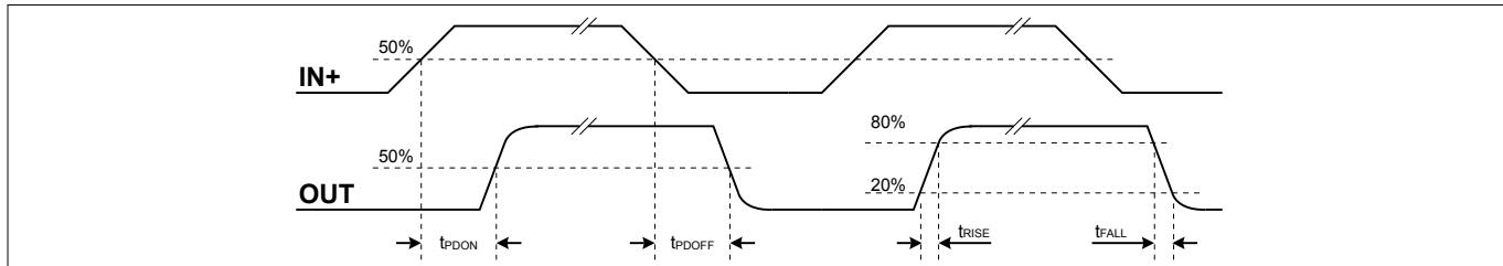
**Figure 8 Propagation delay, rise and fall time**
