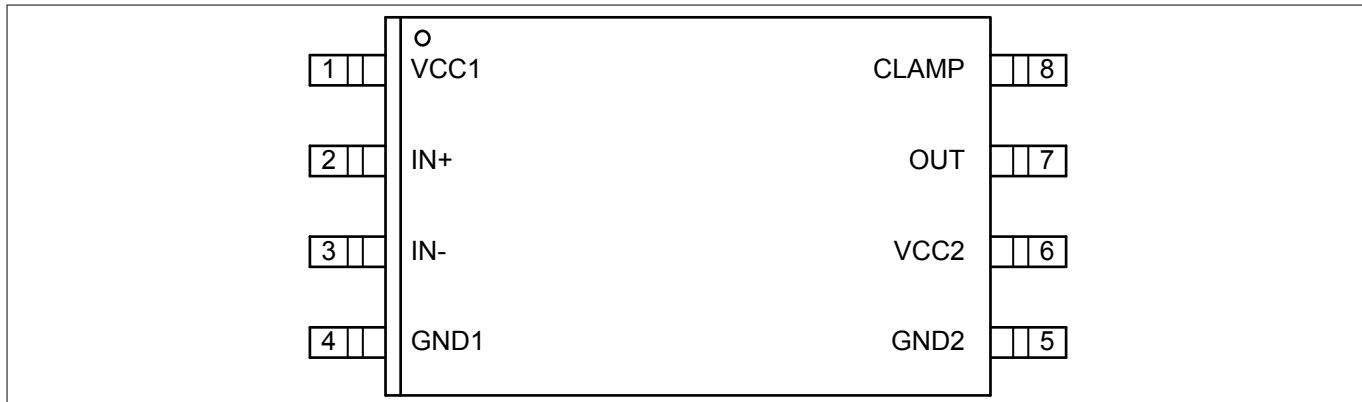
**Figure 3 PG-DSO-8-59 (top view)**
