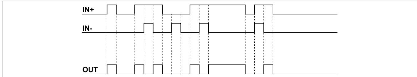
**Figure 6 Logic input to output switching behavior**
