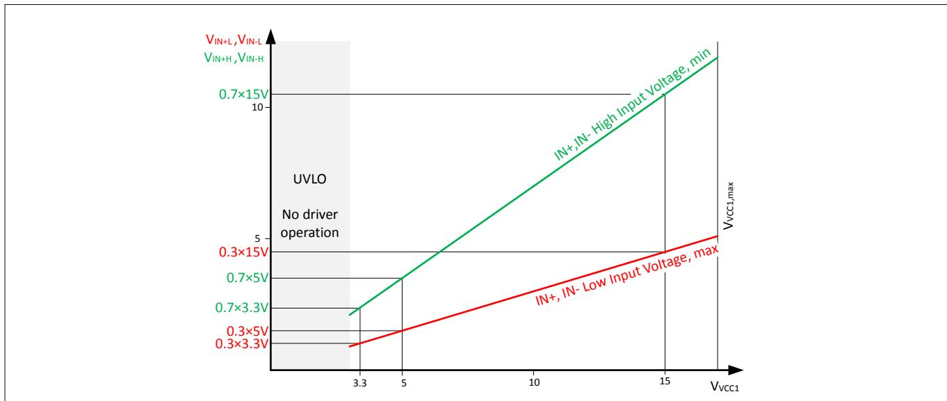
Figure 7  $V_{VCC1}$  scaled input threshold voltage of  $IN+$  and  $IN-$
