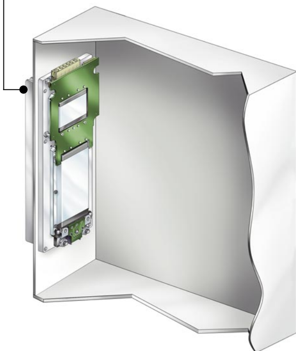
VIPAC with external user supplied heat sink
