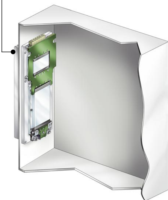
VIPAC with external user supplied heat sink
