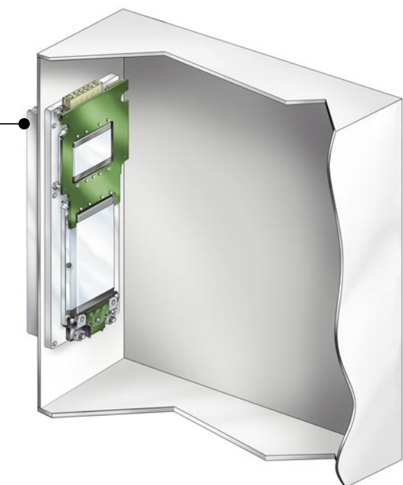
VIPAC with external user supplied heat sink
