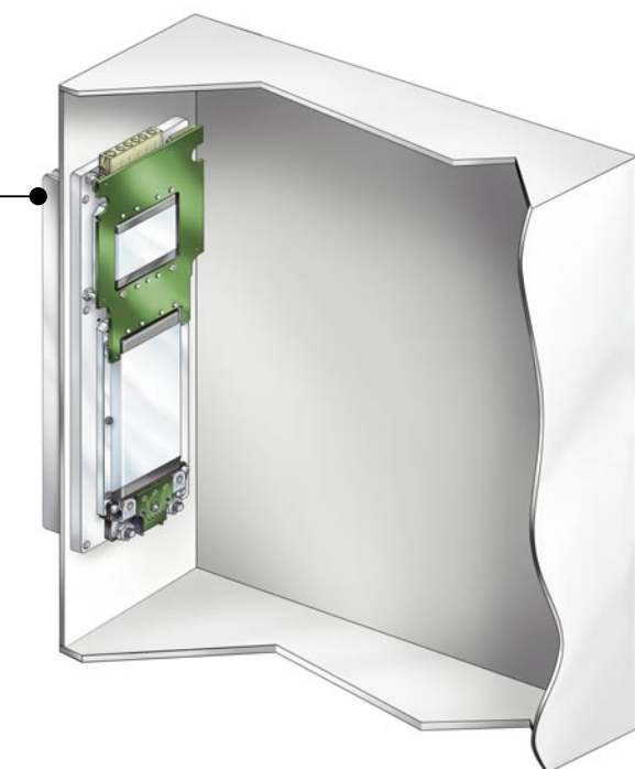
VIPAC with external user supplied heat sink
