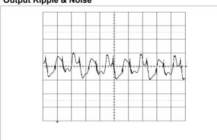
Output voltage ripple at:  $T_{ref}$  = +25°C,  $V_{I}$  = 53 V,  $I_{O}$  = 8.3 A resistive load.
