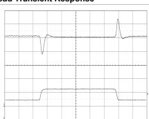
Output voltage response to load current stepchange (2.1-6.2-2.1 A) at: Top trace: output voltage (1.0 V/div.). Bottom trace: load current (5 A/div.). Time scale: (0.1 ms/div.).
