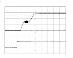
Start-up enabled by connecting V<sub>1</sub> at:  $T_{ref} = +25^{\circ}C$ ,  $V_{l} = 53 V$ ,  $I_{O} = 12.4$  A resistive load.
