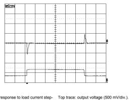
Output voltage response to load current stepchange (3-6-3 A) at: T<sub>ref</sub> =+25°C, V<sub>I</sub> = 53 V.
