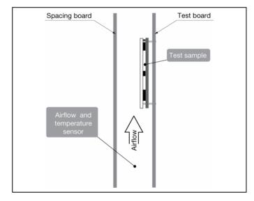
For products with base plate used in a sealed box/cold wall application, cooling is achieved mainly by conduction throughthe cold wall. The Output Current Derating graphs are found in the Output section for each model. The product is tested in a sealed box test set up with ambient temperatures 85, 55 and 35°C. See Design Note 028 for further details.
