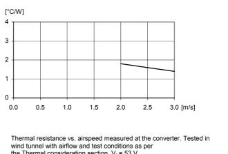
the Thermal consideration section.  $V_1$  = 53 V.
