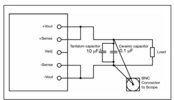
Output ripple and noise test setup
