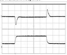
Output voltage response to load current step-change (3.1-9.3-3.1 A) at:  $T_{ref} = +25^{\circ}C$ ,  $V_1 = 53 \text{ V}$
