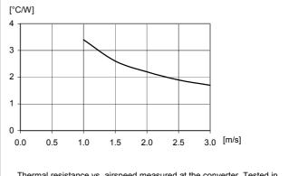
Thermal resistance vs. airspeed measured at the converter. Tested in wind tunnel with airflow and test conditions as per the Thermal consideration section.  $V_1 = 53 \text{ V}$ .
