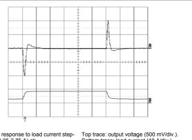
Output voltage response to load current stepchange (2.75-8.25-2.75 A) at: T<sub>ref</sub> =+25°C, V<sub>I</sub> = 53 V.
