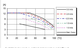
Available load current vs. ambient air temperature and airflow at  $V_1$  = 53 V. See Thermal Consideration section.
