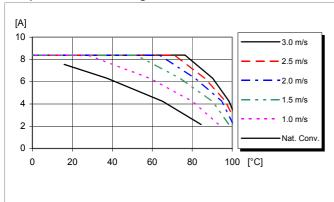
Available load current vs. ambient air temperature and airflow at  $V_{\rm l}$  = 53 V. See Thermal Consideration section.
