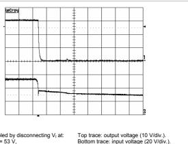
Shut-down enabled by disconnecting V<sub>I</sub> at:  $T_{ref}$  = +25°C, V<sub>I</sub> = 53 V, I<sub>O</sub> = 8.3 A resistive load.
