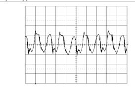
Output voltage ripple at:  $T_{ref}$  = +25°C,  $V_I$  = 53 V,  $I_O$  = 12.4 A resistive load.
