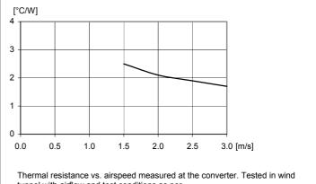
Thermal resistance vs. airspeed measured at the converter. Tested in wind tunnel with airflow and test conditions as per the Thermal consideration section.  $V_l = 53 \text{ V}$ .
