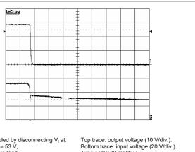
Shut-down enabled by disconnecting  $V_{l}$  at:  $T_{ref}$  = +25°C,  $V_I$  = 53 V,  $I_O$  = 11 A resistive load.
