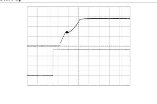
Start-up enabled by connecting V<sub>1</sub> at:  $T_{ref} = +25^{\circ}C$ ,  $V_{I} = 53 V$ ,  $I_{O} = 8.3 A$  resistive load.
