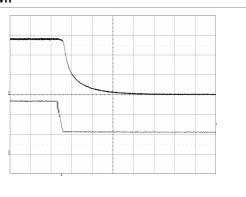
Shut-down enabled by disconnecting  $V_i$  at:  $T_{ref}$  = +25°C,  $V_I$  = 53 V,  $I_O$  = 8.3 A resistive load.
