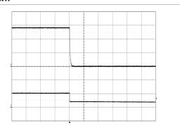
Shut-down enabled by disconnecting V<sub>1</sub> at:  $T_{ref}$  = +25°C,  $V_I$  = 53 V,  $I_O$  = 12.4 A resistive load
