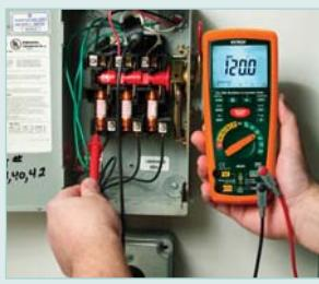
Only a True RMS meter can give accurate readings of distorted waveforms
