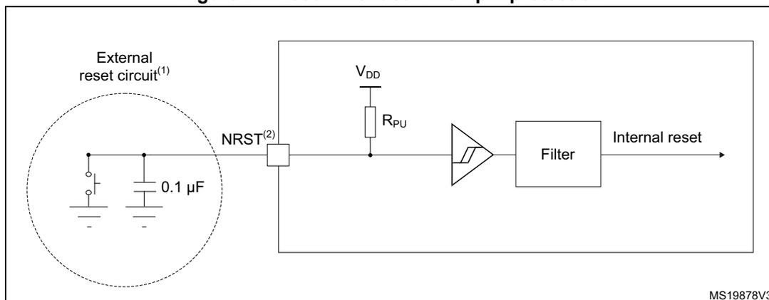
1. The reset network protects the device against parasitic resets.
