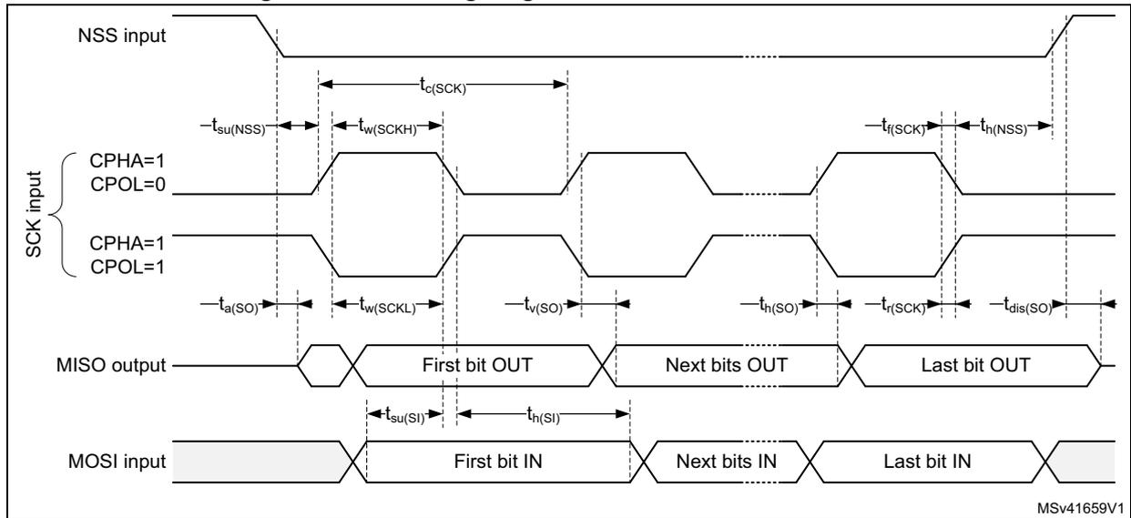
1. Measurement points are done at CMOS levels: 0.3 V<sub>DD</sub> and 0.7 V<sub>DD</sub>.
