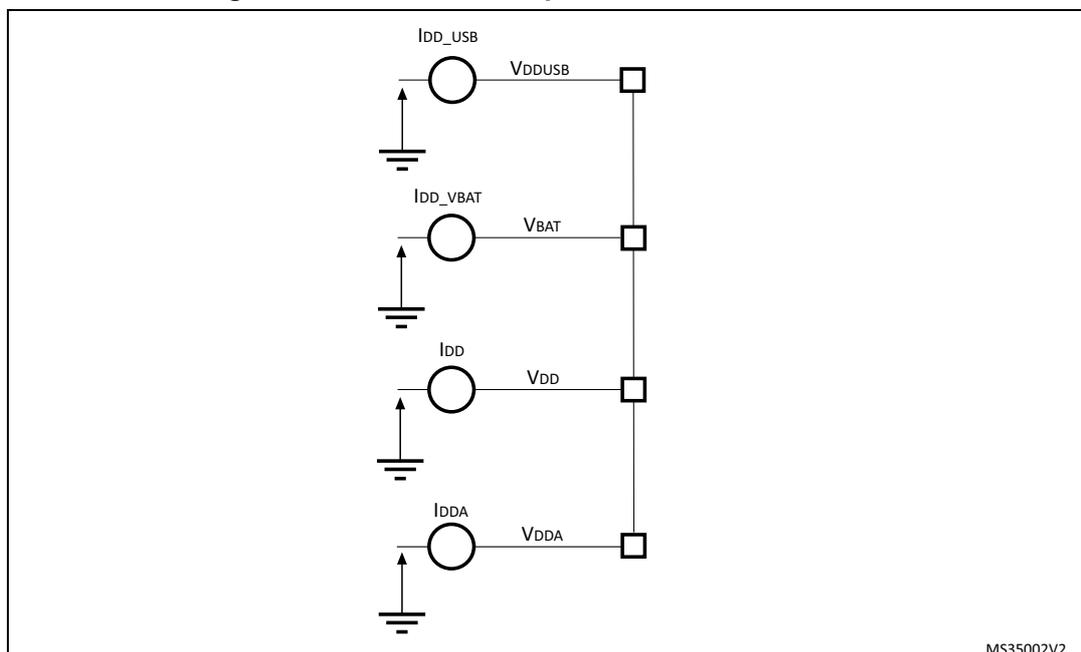
The  $I_{DD\_ALL}$  parameters given in [Table 26](#) to [Table 38](#) represent the total MCU consumption including the current supplying  $V_{DD}$ ,  $V_{DDA}$ ,  $V_{DDUSB}$  and  $V_{BAT}$ .
