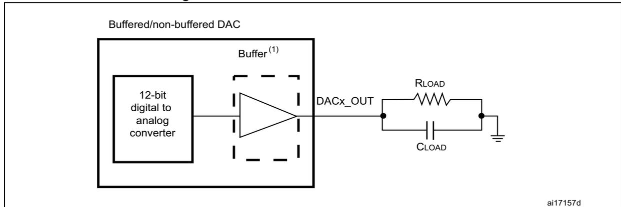
1. The DAC integrates an output buffer that can be used to reduce the output impedance and to drive external loads directly without the use of an external operational amplifier. The buffer can be bypassed by configuring the BOFFx bit in the DAC\_CR register.
