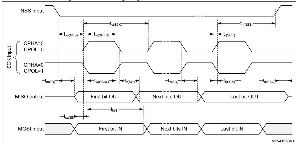
Figure 32. SPI timing diagram - slave mode and CPHA = 1
