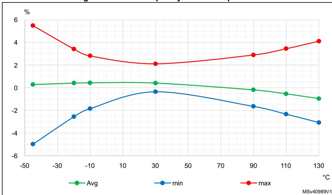
Low-speed internal (LSI) RC oscillator
