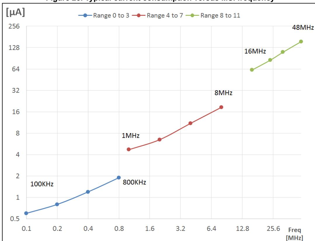
High-speed internal 48 MHz (HSI48) RC oscillator
