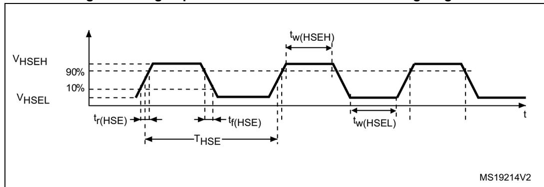
**Low-speed external user clock generated from an external source**
