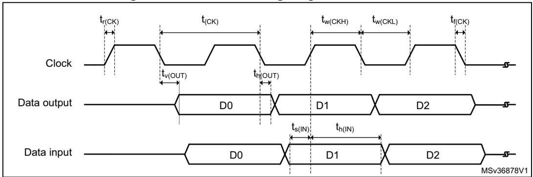
Figure 35. Quad SPI timing diagram - DDR mode
