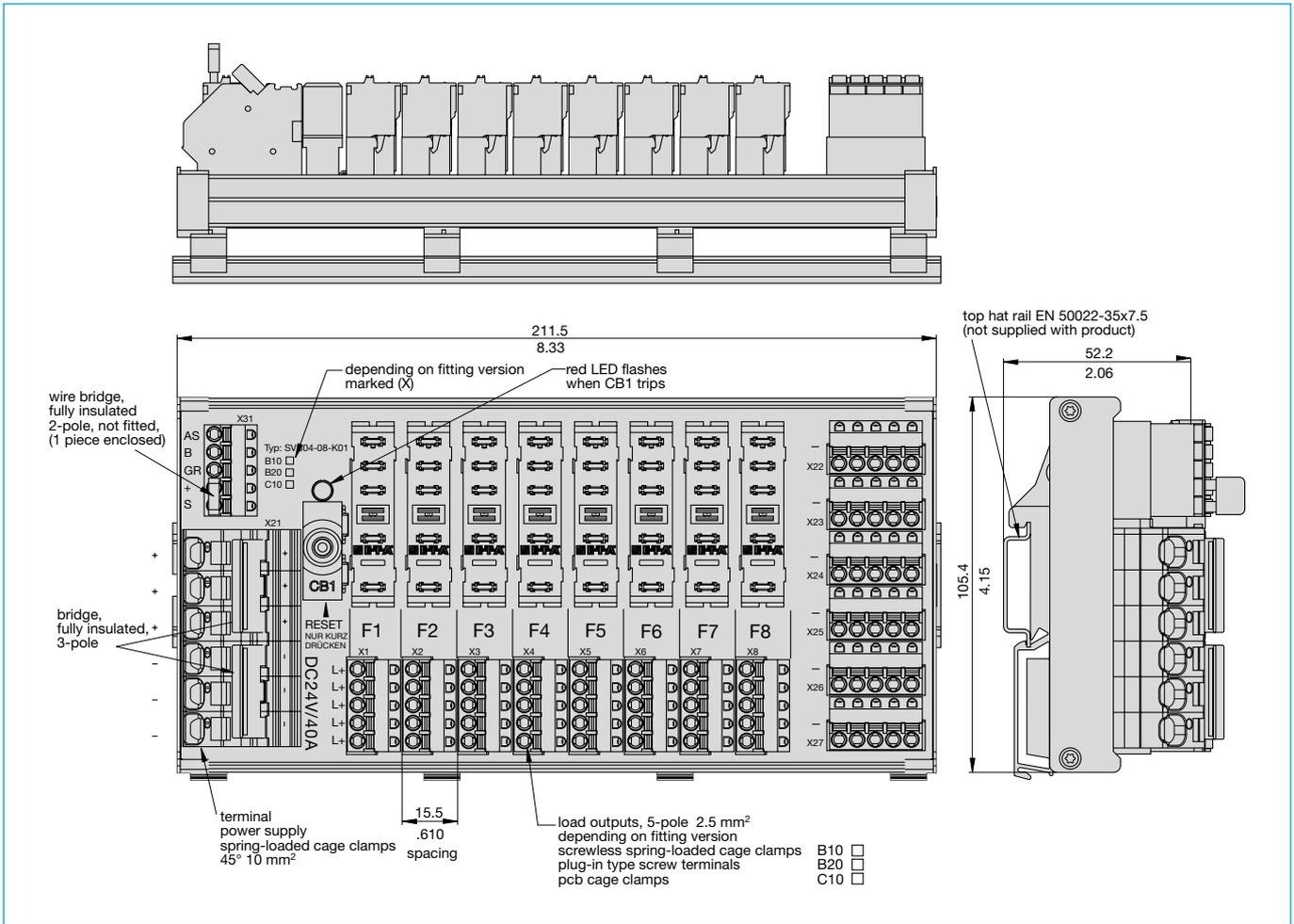
**Schematic diagram SVS04-08... K01 (fitted with ESS20-003)**
