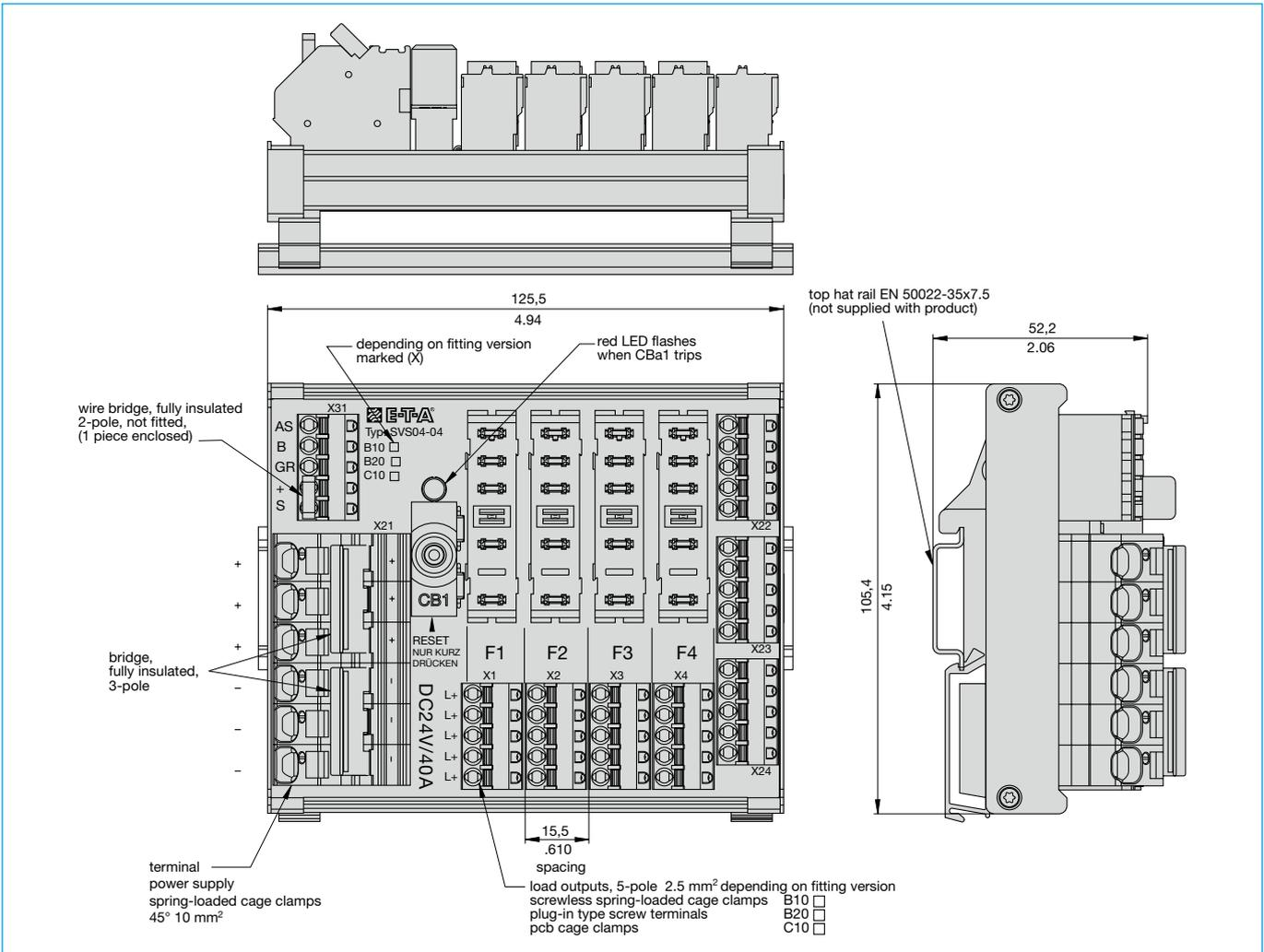
**Schematic diagram SVS04-04-... (fitted with ESS20-003)**
