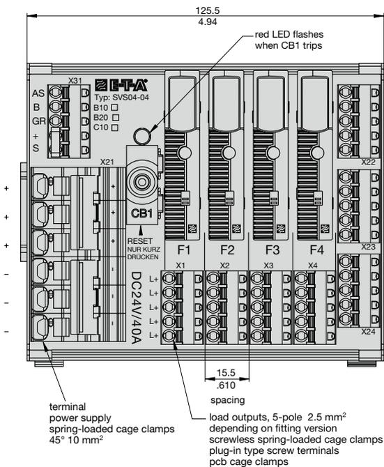
terminal power supply spring-loaded cage clamps 45° 10 mm<sup>2</sup>
