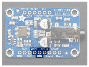
Three pins are used for stereo I2S data in. These pins are required!
