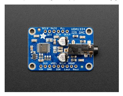
For inputs, you can use classic I2S (the default) or 16-bit, 20-bit or 24-bit left justified data. You can set it up to take an input system/main clock but we default-set it to just generate it for you, so you only need to connect Data In, Word Select (Left/Right Clock) and Bit Clock lines. If you want, there's a mute pin and a de-emphasis filter you can turn on.
