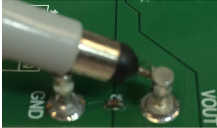
Figure 3. Output Ripple Measurement Technique
