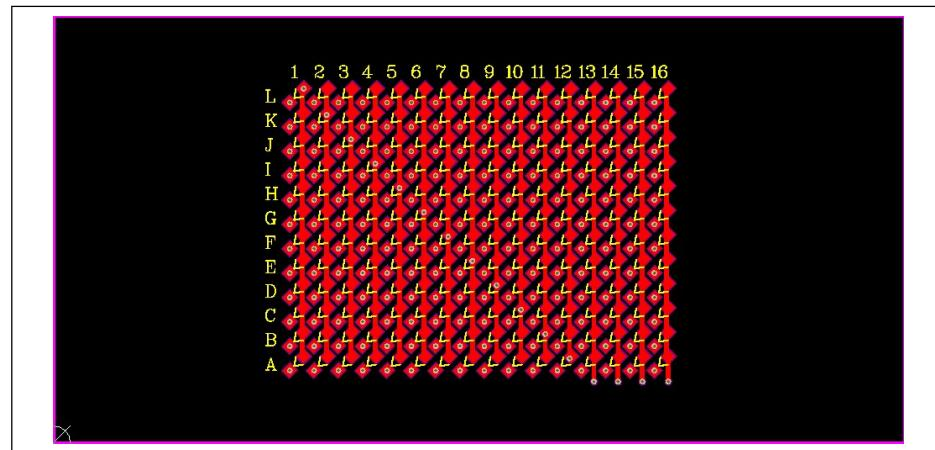
Figure 8: LED Board PCB Layout - Top Layer
