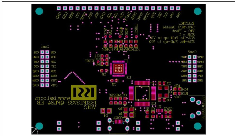
Figure 5: Board Component Placement Guide - Bottom Layer
