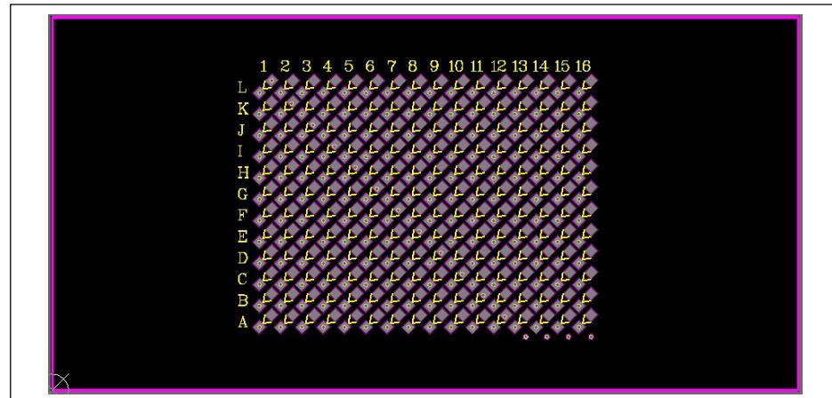
Figure 7: LED Board Component Placement Guide - Top Layer
