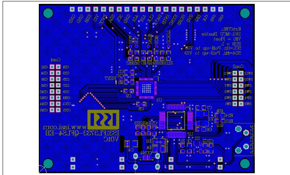
Figure 6: Board PCB Layout - Bottom Layer
