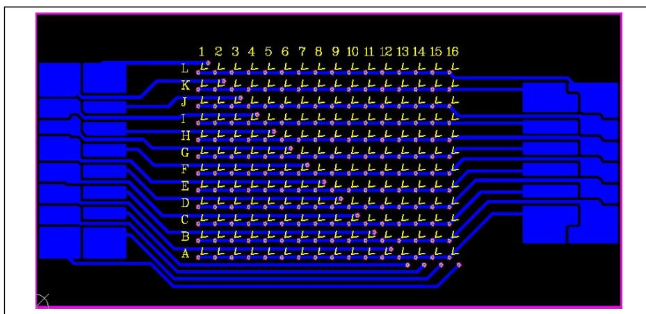
Figure 10: LED Board PCB Layout - Bottom Layer
