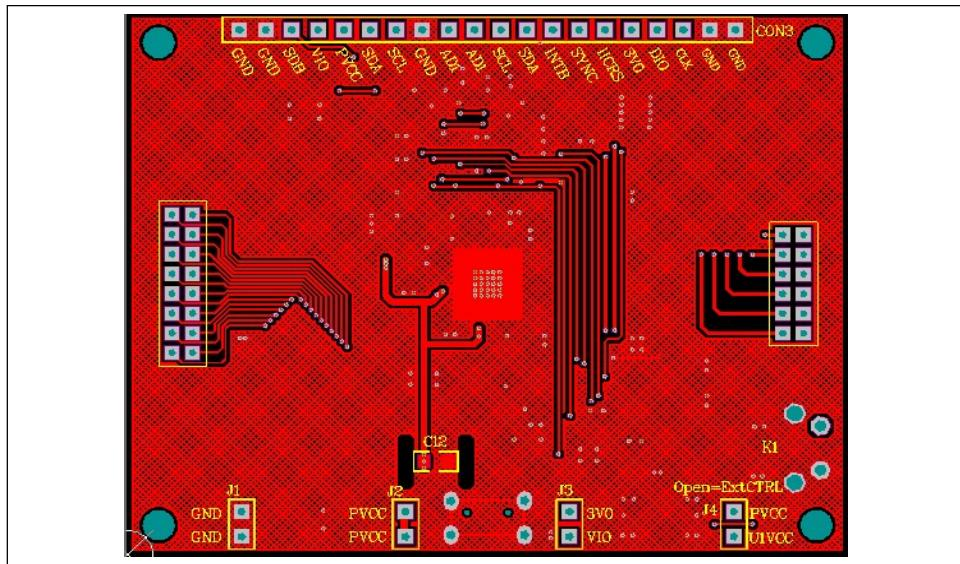
Figure 4: Board PCB Layout - Top Layer
