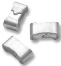
A range of unique surface mount devices. Avoid damage to sensitive tiny electronic circuits by incorporating these probe pads in the circuitry. A choice of three sizes relate to standard chip footprint areas. These probe pads are packaged on tape for high speed automatic placement. They enable safe probing of circuitry when adjusting, setting up measuring or repairing tiny electronic circuitry.
