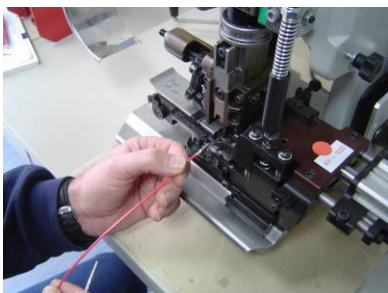
The picture shows crimping process with Mini-applicator
