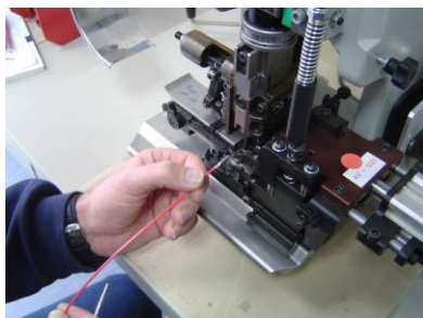
The picture shows crimping process with Mini-applicator
