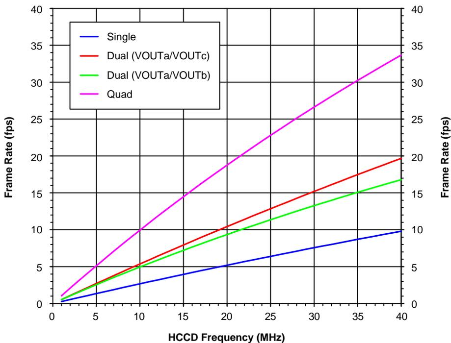
Figure 20. Frame Rates – 1/4 Resolution – Variable HCCD XLDR
