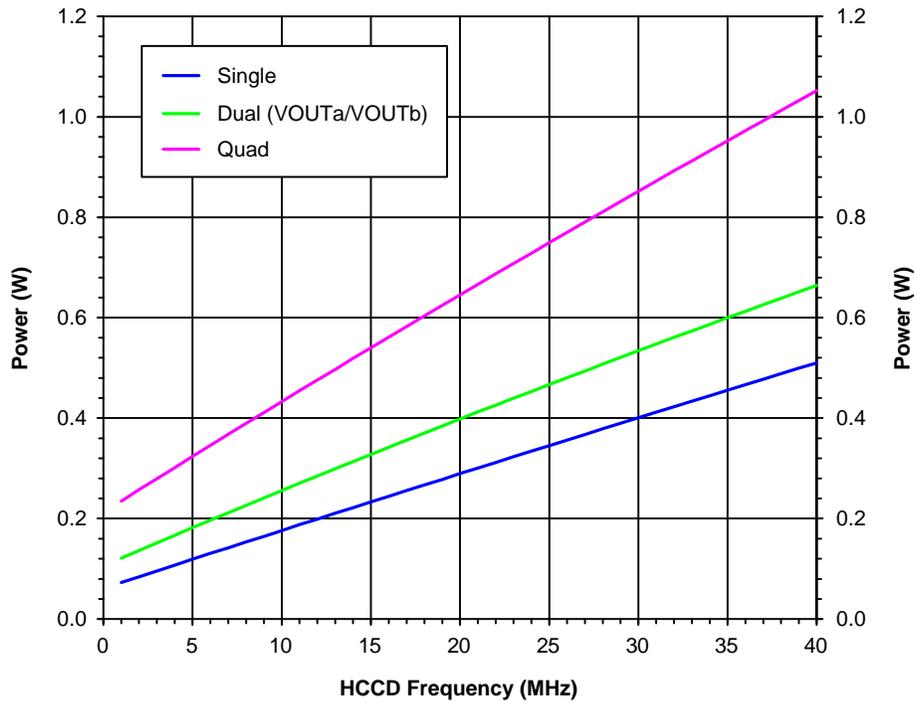
Figure 15. Power – 1/4 Resolution – Constant HCCD
