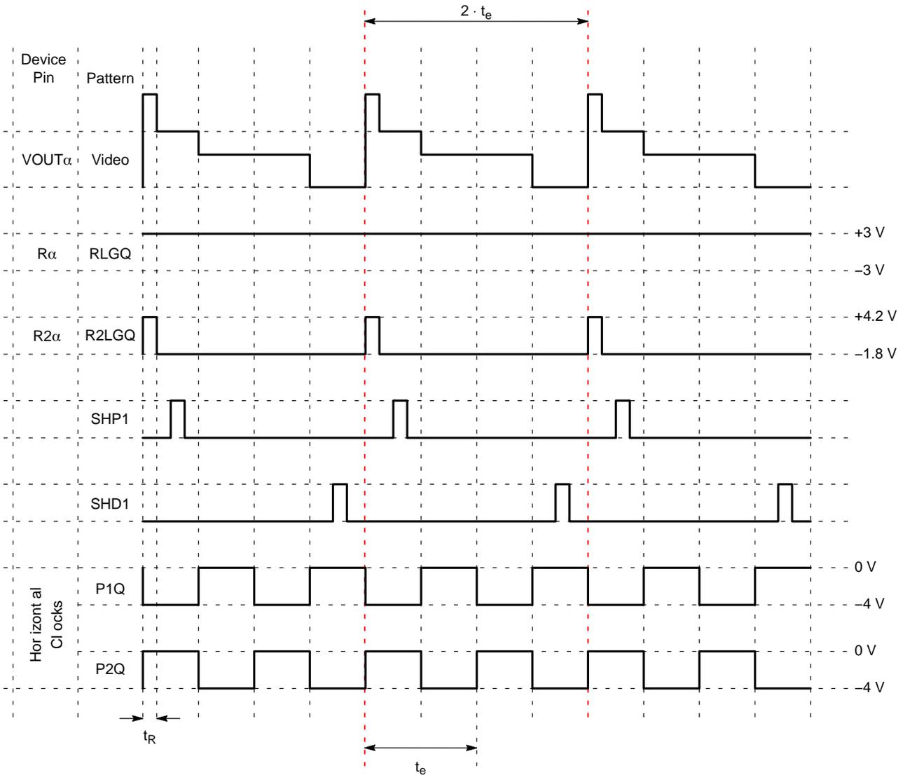
**Figure 43. Pixel Timing Diagram – 1/4 Resolution – Low Gain**
