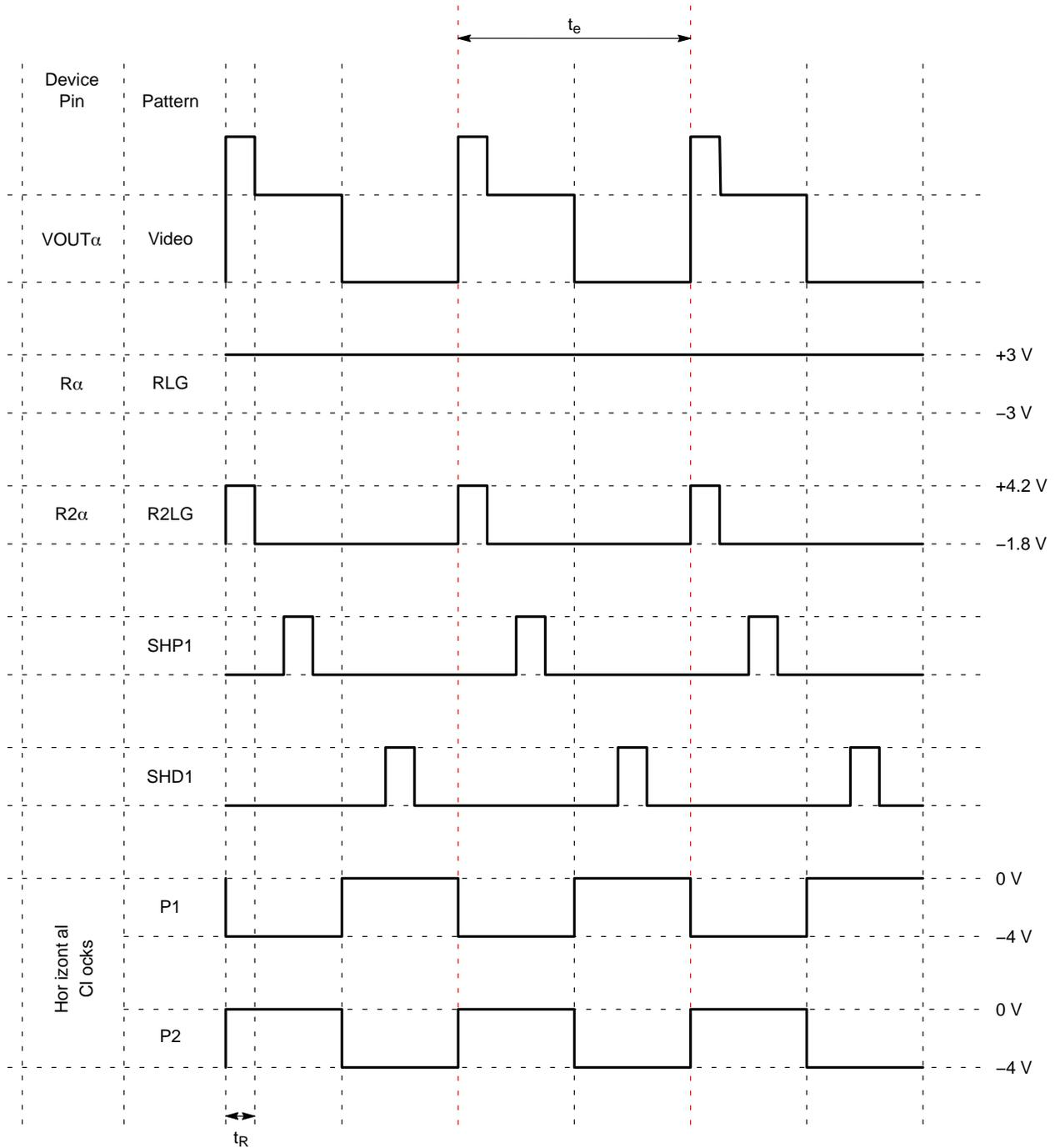
Figure 41. Pixel Timing Diagram – Full Resolution – Low Gain
