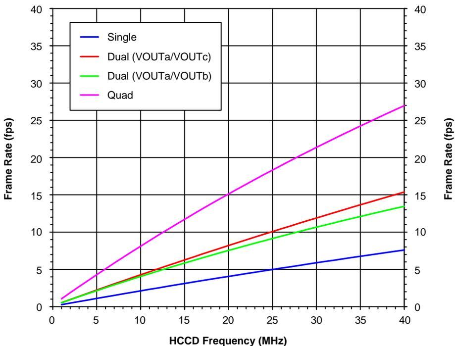
Figure 21. Frame Rates – 1/4 Resolution – Constant HCCD XLDR
