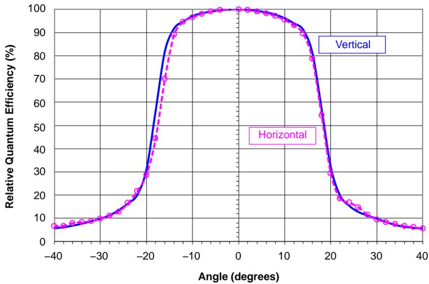
Figure 11. Monochrome with Microlens Angular Quantum Efficiency
