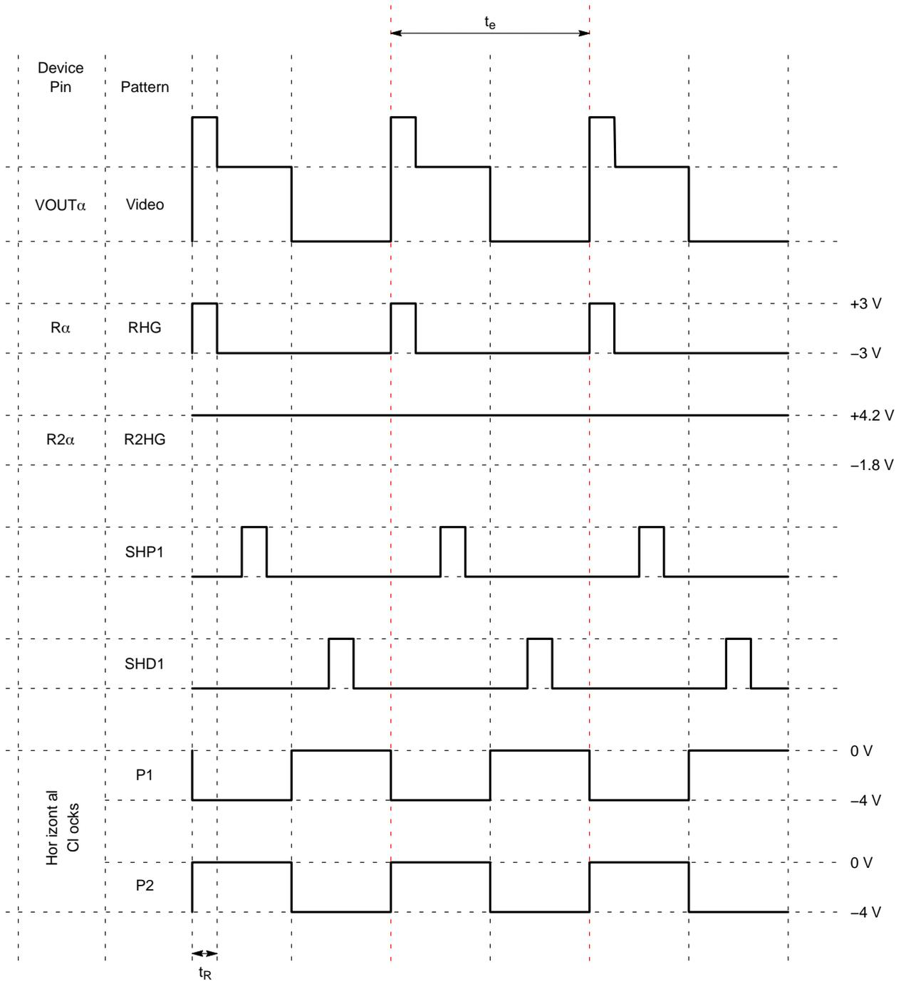
Figure 40. Pixel Timing Diagram – Full Resolution – High Gain
