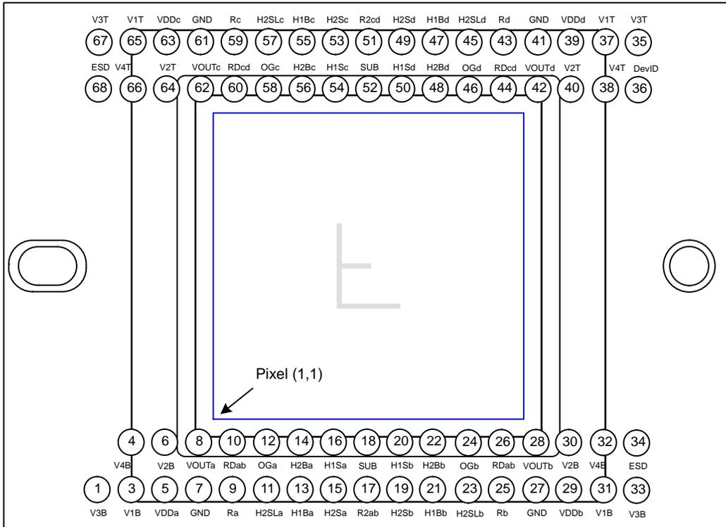
Figure 5. Package Pin Designations – Top View
