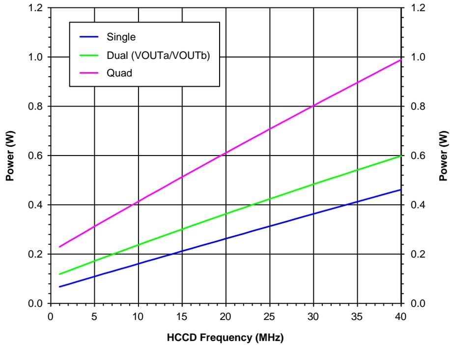
Figure 16. Power – 1/4 Resolution – Variable HCCD XLDR
