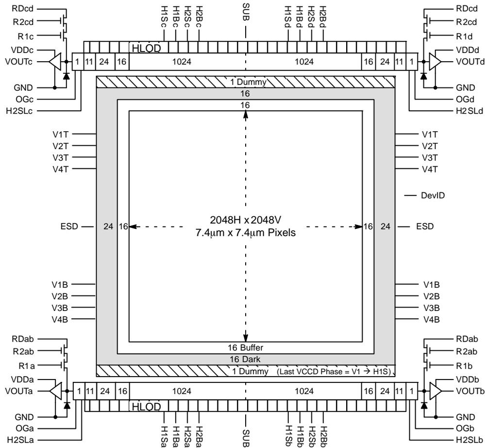
Figure 2. Block Diagram
