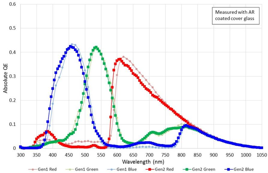
Figure 9. Color (Bayer RGB) with Microlens Quantum Efficiency
