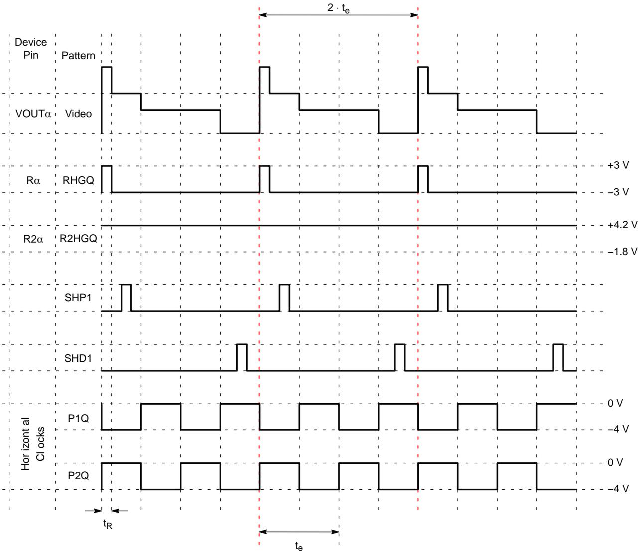
**Figure 42. Pixel Timing Diagram – 1/4 Resolution – High Gain**
