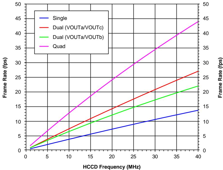
Figure 19. Frame Rates – 1/4 Resolution – Constant HCCD
