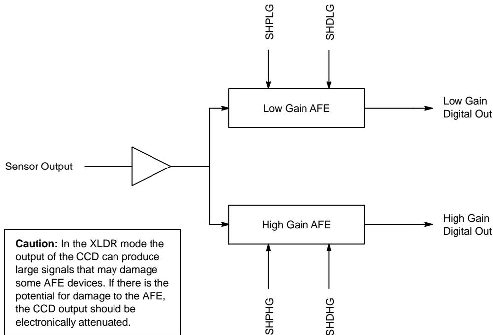
Figure 44. XLDR Timing – AFE Connections Block Diagram
