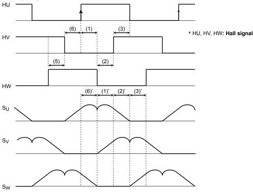
In the above diagram, the modulated waveforms have an interval (1)' that is equal to the interval between a rising edge of HU to a falling edge of HW (1) of the previous cycle. In the same way, the modulated waveforms have an interval (2)' that is equal to the interval between a falling edge of HW to a rising edge of HV (2) of the previous cycle. If there is not a next edge before 32 ticks end, next 32 ticks become equal to the next period until the next edge.
