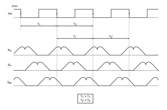
In the above diagram, the modulated waveforms have an interval (T1') that is equal to the interval between a falling edge of HU to its next falling edge (T1) of the previous cycle. If there is not an HU falling edge before T1' ends, T2' becomes equal to T1' until the next falling edge of HU.
