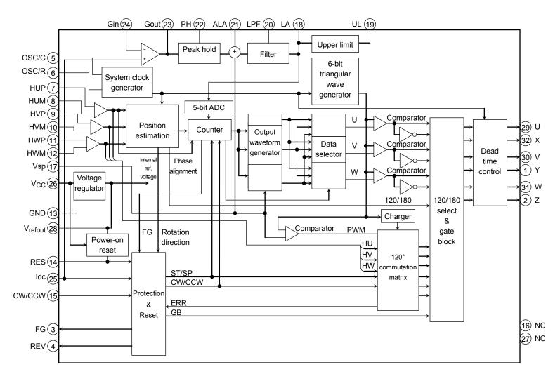
Some of the functional blocks, circuits, or constants in the block diagram may be omitted or simplified for explanatory purposes.
