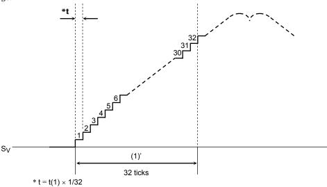
Phase matching between the hall signal and the modulated waveform is carried out for every zero cross of the hall signal.
