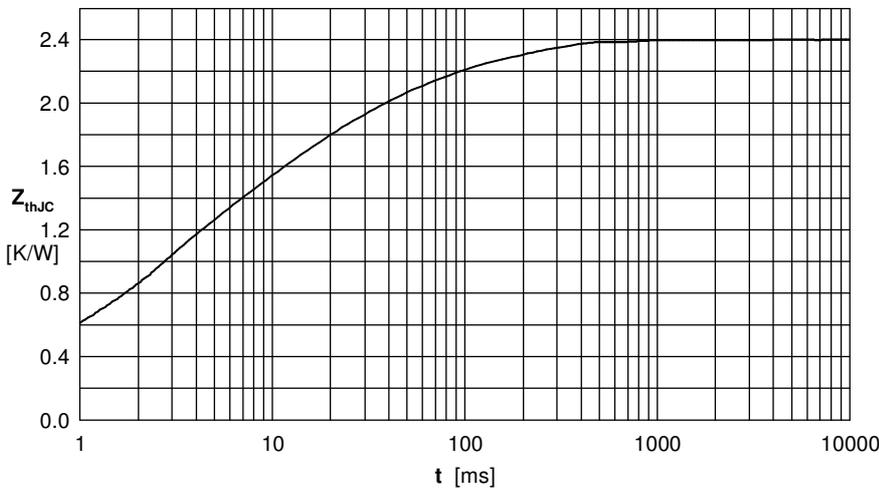
Fig. 6 Transient thermal impedance junction to case
