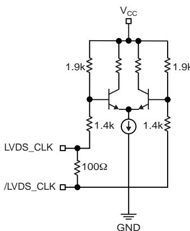
Figure 2. Simplified LVDS Input Stage
