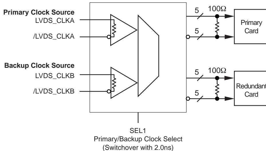
System using SY89828L as a switchover circuit from a Primary Clock to a Redundant backup Clock in a fail-safe application.
