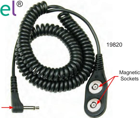
Jewel® MagSnap Coil Cords meet or exceed the requirements of ANSI/ESD S20.20 and ANSI/ESD S1.1 including section 5.4 Breakaway Force "With the ground cord connected to the cuff in a normal manner, a force of  $\geq .45$  kg (1 lb) but  $\leq 2.3$  kg (5 lb) applied to the ground cord, in the normal disconnect direction, shall be required to separate the ground cord from the cuff."
