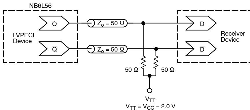
**Figure 16. Typical Termination for LVPECL Output Driver and Device Evaluation
