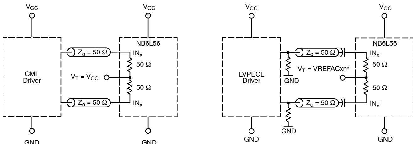
Figure 14. Typical Standard  $50 \Omega$  Load CML Interface
