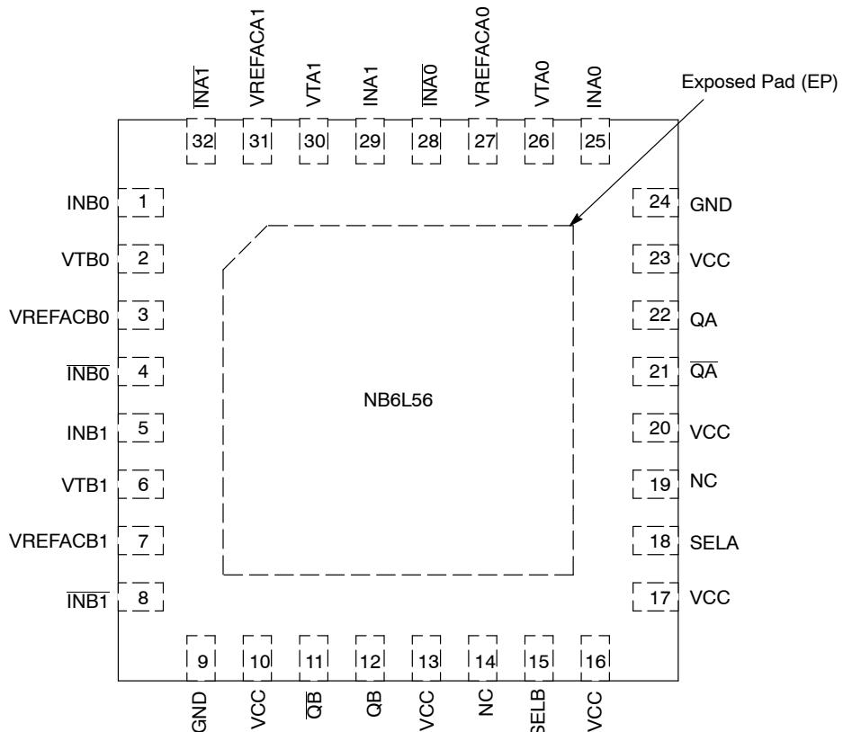
**Figure 3. NB6L56 Pinout: QFN-32 (Top View)**
