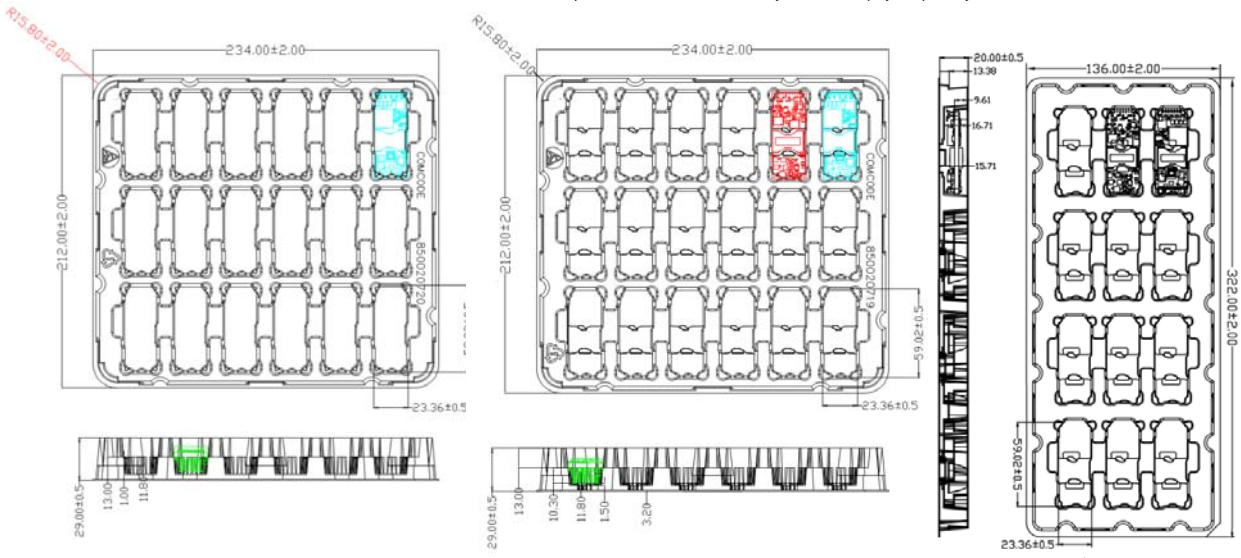
Open Frame Through Hole Pin Module Tray Figure 27. EBDW020 Packaging Tray
