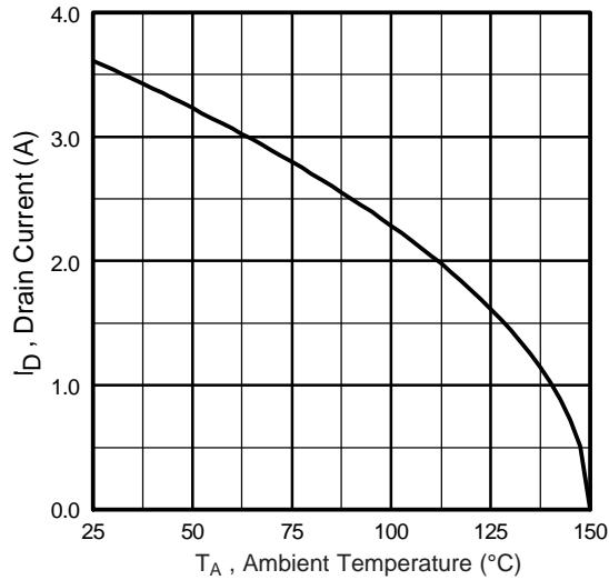
**Fig 9.** Maximum Drain Current Vs.
