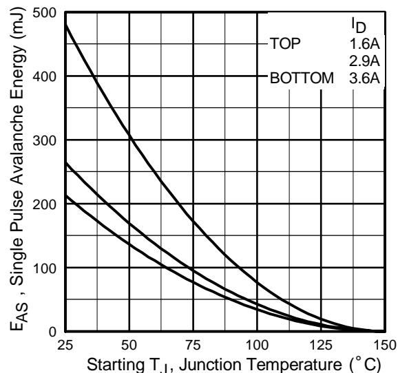
**Fig 14c.** Maximum Avalanche Energy Vs. Drain Current
