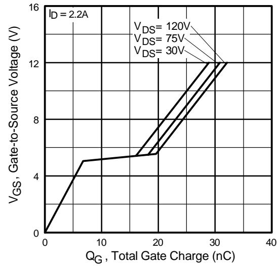
**Fig 6.** Typical Gate Charge Vs.
