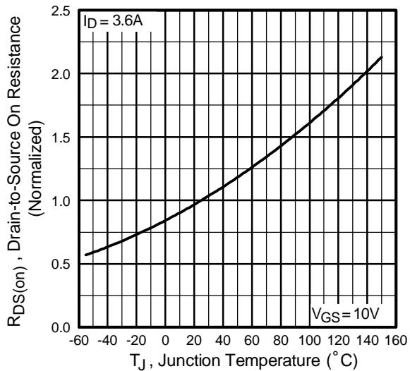
**Fig 4.** Normalized On-Resistance
