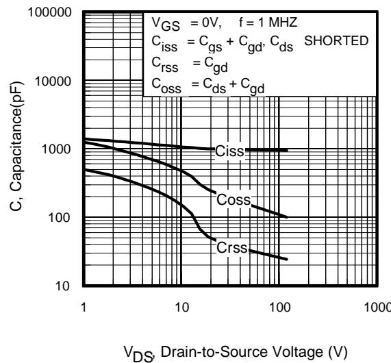
**Fig 5.** Typical Capacitance Vs.
