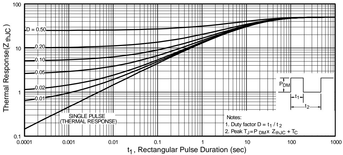
**Fig 10.** Maximum Effective Transient Thermal Impedance, Junction-to-Case
