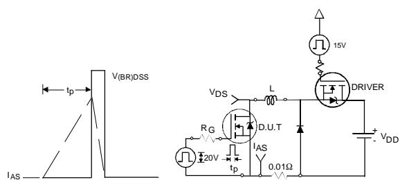
**Fig 14a&b.** Unclamped Inductive Test circuit and Waveforms
