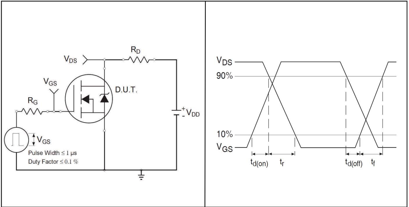
Figure 24a Switching Time Test Circuit
