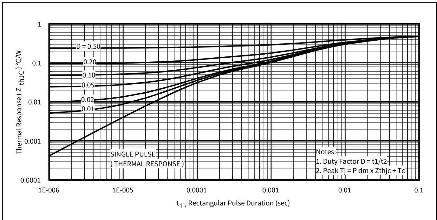
**Figure 15** Maximum Effective Transient Thermal Impedance, Junction-to-Case
