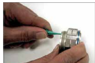
Plastic tool with contact in proper position.
