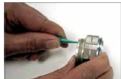
Plastic tool with contact in proper position.
