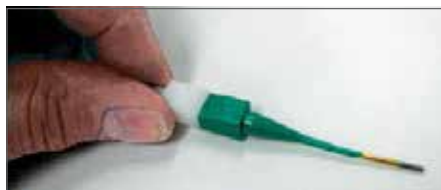
Plastic tool with contact in proper position.
