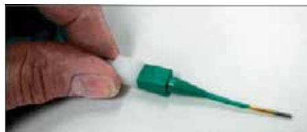
Plastic tool with contact in proper position.
