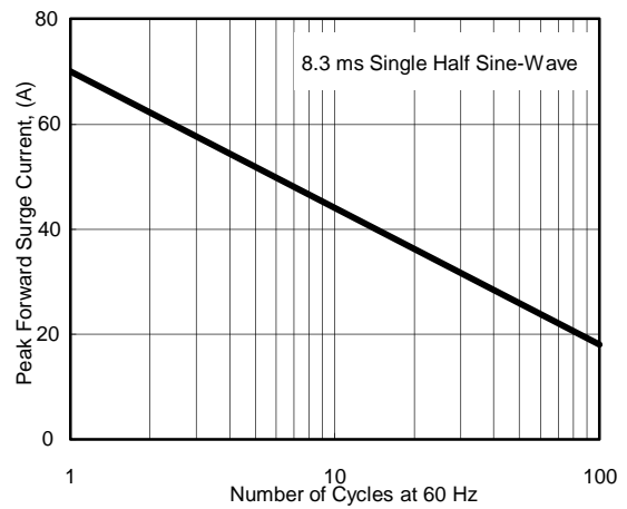
Fig. 2 - Maximum Non-Repetitive Surge Current
