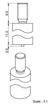
Technical Tolerances according to DIN ISO 2768m In tape & reel packaging a cap is fixed to the product to realize automatic assembly
