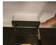
Fasten the 2 screws to fix the peripheral in place
