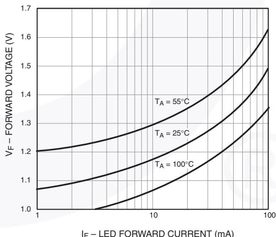
**Figure 8. LED Forward Voltage vs. Forward Current**
