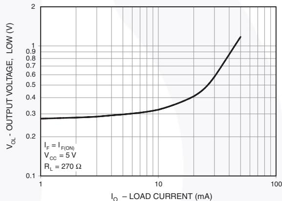
**Figure 6. Output Voltage, Low vs. Load Current**
