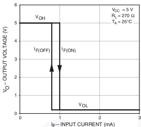
**Figure 3. Transfer Characteristics**
