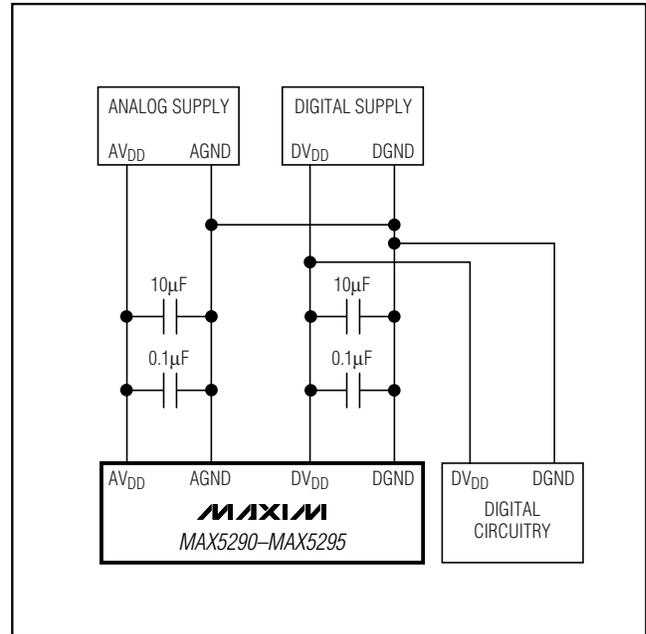
Figure 11. Separate Analog and Digital Power Supplies
