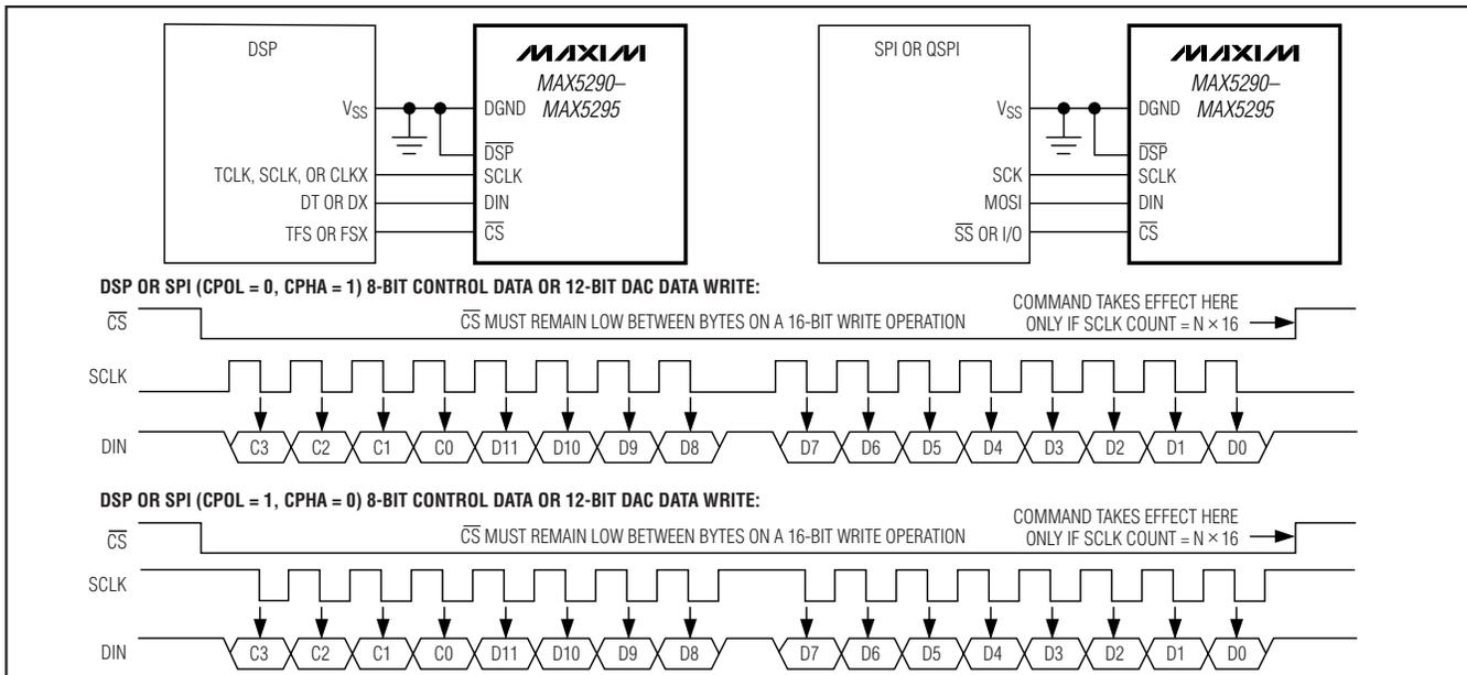
Figure 4. DSP and SPI (CPOL = 0, CPHA = 1 or CPOL = 1, CPHA = 0) DAC Writes
