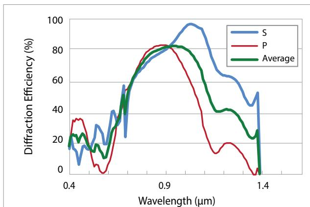
Typical absolute diffraction efficiency at AOI 61.2° \*
