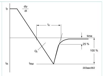
Fig. 6. Reverse recovery definitions; ramp recovery
