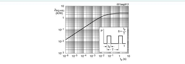
Fig. 4. Transient thermal impedance from junction to mounting base as a function of pulse width
