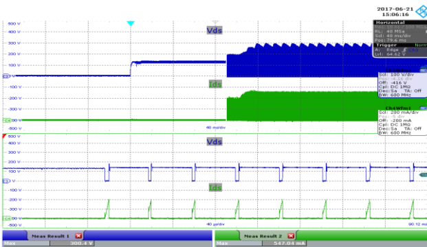
Figure 30 – Drain Voltage and Current Waveforms. 90 VAC Input, Full Load. Upper: V_{DRAIN} , 100 V, 40 ms, 40 \mu s / div. Lower: I_{DRAIN} , 200 mA / div.
