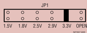
Figure 2. Output Voltage Selection (JP1) (3.3V Position Shown)
