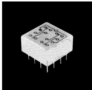
This .150 four pole double throw Grid-space relay is the companion to the two pole 3SBC type shown on page 1-41. It also features the same .150 inch pin spacing that allows you to insert the relay with no intermediate pin spreaders. There is adequate clearance for conductors to reach all pins. It is a very compact 4 pole double throw 2 ampere relay.
