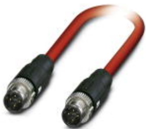
Assembled Sercos III cable, shielded, star quad, 22 AWG stranded (7-wire), RAL 3020 (traffic red), M12 plug, SPEEDCON, 4-pos. to M12 plug, SPEEDCON, length: 0.5 m
