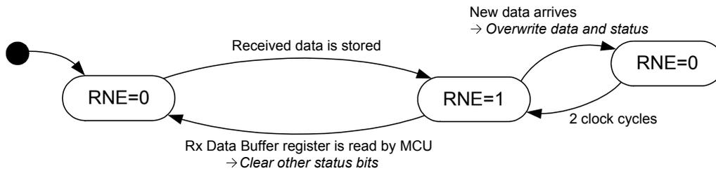
**Figure 23. Periodic data collection mode RNE bit behavior**
