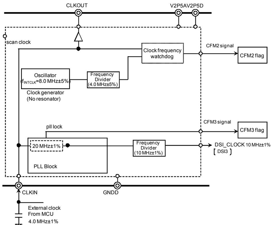
**Figure 25. Clock module pins and block diagram**
