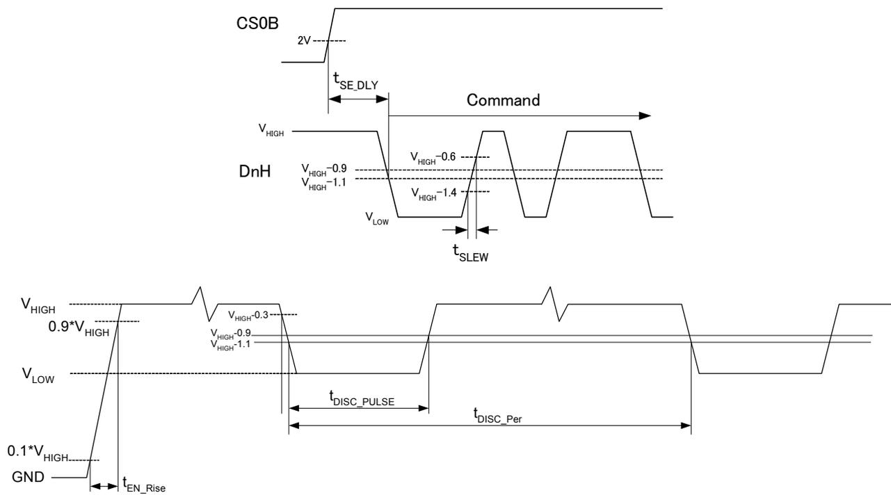
Figure 11. DSI bus voltages timings
