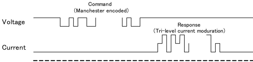
Figure 15. DSI Command and response mode operating principle
