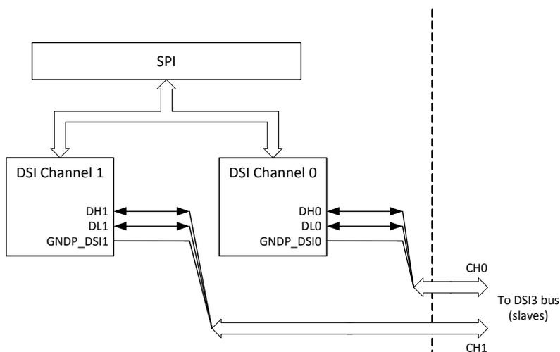
**Figure 9. DSI modules pins and block diagram**
