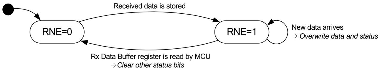
Figure 17. Command and response mode RNE bit behavior
