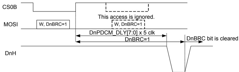
**Figure 21. Periodic data collection mode manual BRC**
