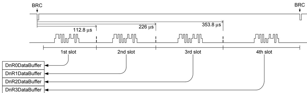
Figure 19. DSI periodic data collection mode operating principle
