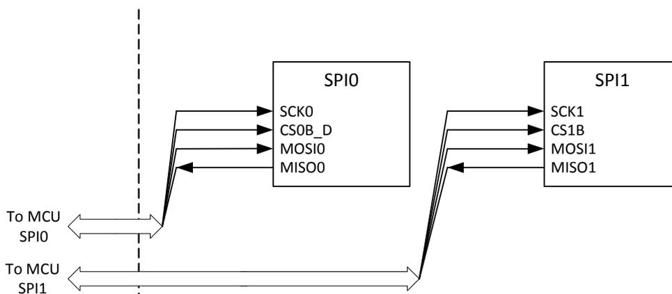
Figure 5. SPI modules pins and block diagram
