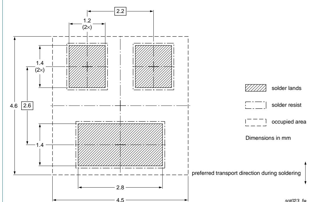
Fig 19. Wave soldering footprint PDTA143ZT (SOT23)
