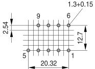
Hole arrangement View in mounting direction
