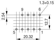
Hole arrangement View in mounting direction
