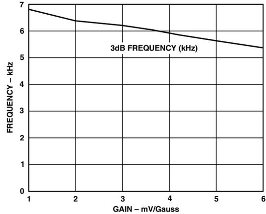
Figure 13. Small Signal Gain Bandwidth vs. Gain
