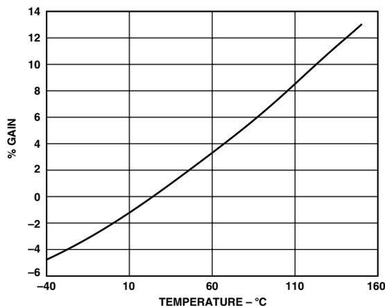
Figure 4. Uncompensated Gain Variation (from  $25^{\circ}\text{C}$ ) vs. Temperature
