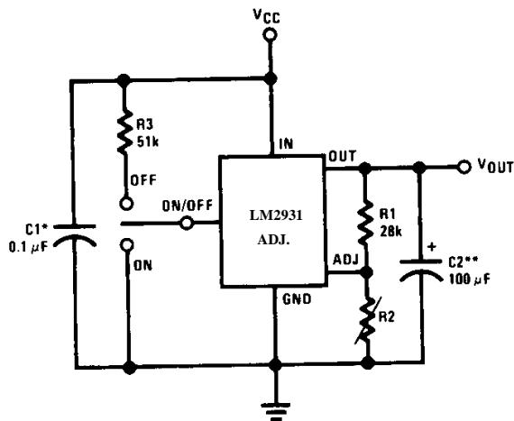
$$V_{OUT} = \text{Reference Voltage} \times \frac{R_1 + R_2}{R_1}$$
