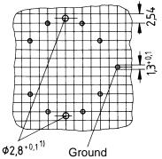
Hole arrangement View in mounting direction
