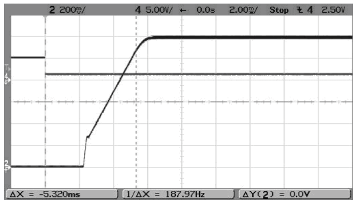
On/Off Enable Startup (V in =5V, V out =1.2V, I out =6A, Cload=0) Trace 4=Enable, Trace 2=Vout
