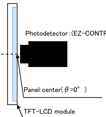
fig.2-1 Measuring method of Viewing angle range.
