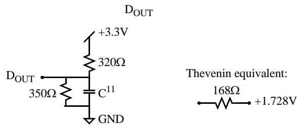
Figure B: 3.3V Output load
