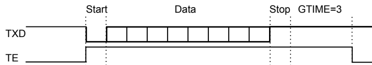
Figure 32-14. Example of TE Drive with Guard Time
