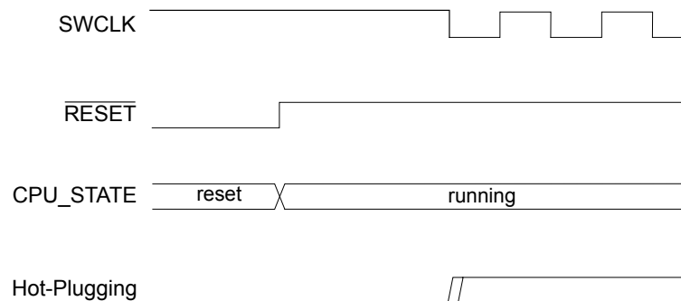
Figure 14-3. Hot-Plugging Detection Timing Diagram
